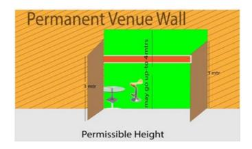
\*4.0 Mtrs. height is only permissible to wall which is towards permanent structure/wall.
